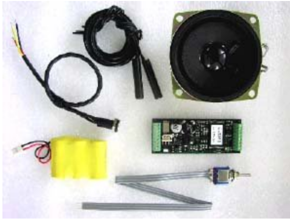
Components of a typical BigSound™ 2K2 diesel kit.
