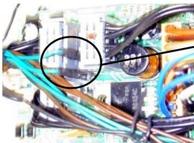
There are two pins labeled “SND” on the LGB circuit board. Slip one of the Phoenix power clips over each pin and connect to terminals 1 & 2 on the 2K2 or PB9. Since this is a DCC situation, polarity will not matter. The P5 can be powered from these pins as well.
