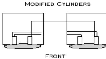
9. Once you have switch contacts that work, you will be getting two chuffs per revolution of the crankshaft. The chuffs will have an uneven pattern because of the quartering of the two flywheels. You must “un-quarter” the flywheels so that the switch contacts are made every 180° of rotation. As-received the flywheels are set 90° apart (quartered). Manually turn the flywheels on either side of the engine until they are offset 180° rather than 90°.
