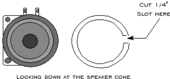
Place the speaker cone down with the mounting holes toward the back of the tender. Locate the two small square holes on the floorboard slats close to the back. Align the back edge of the speaker rim with the floorboard groove that runs through the holes. The speaker should be set so that the floorboard groove is just visible. It is imperative that the speaker is placed precisely in order for
