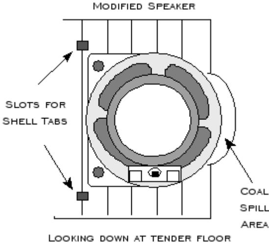
shell to fit back on the tender floor. The front edge of the speaker extends into the area where the coal spill is modeled at the forward end of the tender. Make sure that any loose pieces of the model are glued securely in place. Any extra time you spend making sure you have a good acoustic chamber is well worth the effort. Set the engine aside to allow the adhesive to set.
