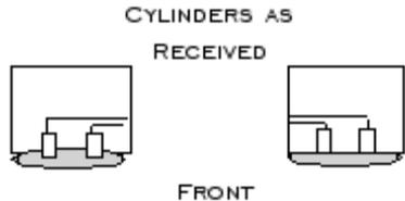
3. Inside the engineer's cylinder box, de-solder the inside wire and solder it to the outside pin, as represented by the dashed line in the sketch.
