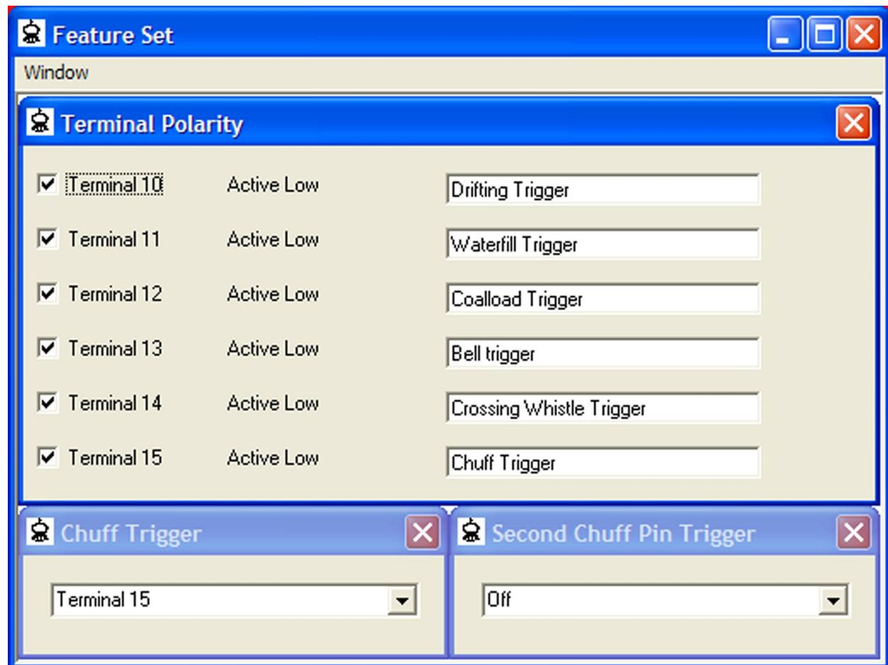
**Chuff [Pin only, Steam]:** Determines the method for deriving speed. Assigning the Pin to a terminal value means that each contact closure produces one chuff cycle – the number of chuffs per closure is set by the Chuff Hits feature which is found under the Chuff Mode icon. A setting of “Auto” means that the system will derive speed from the input voltage.
