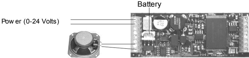
For bench testing, connect the speaker to terminals 7 & 8, plug in the battery, and hook your bench power supply to terminals 1 & 2.
