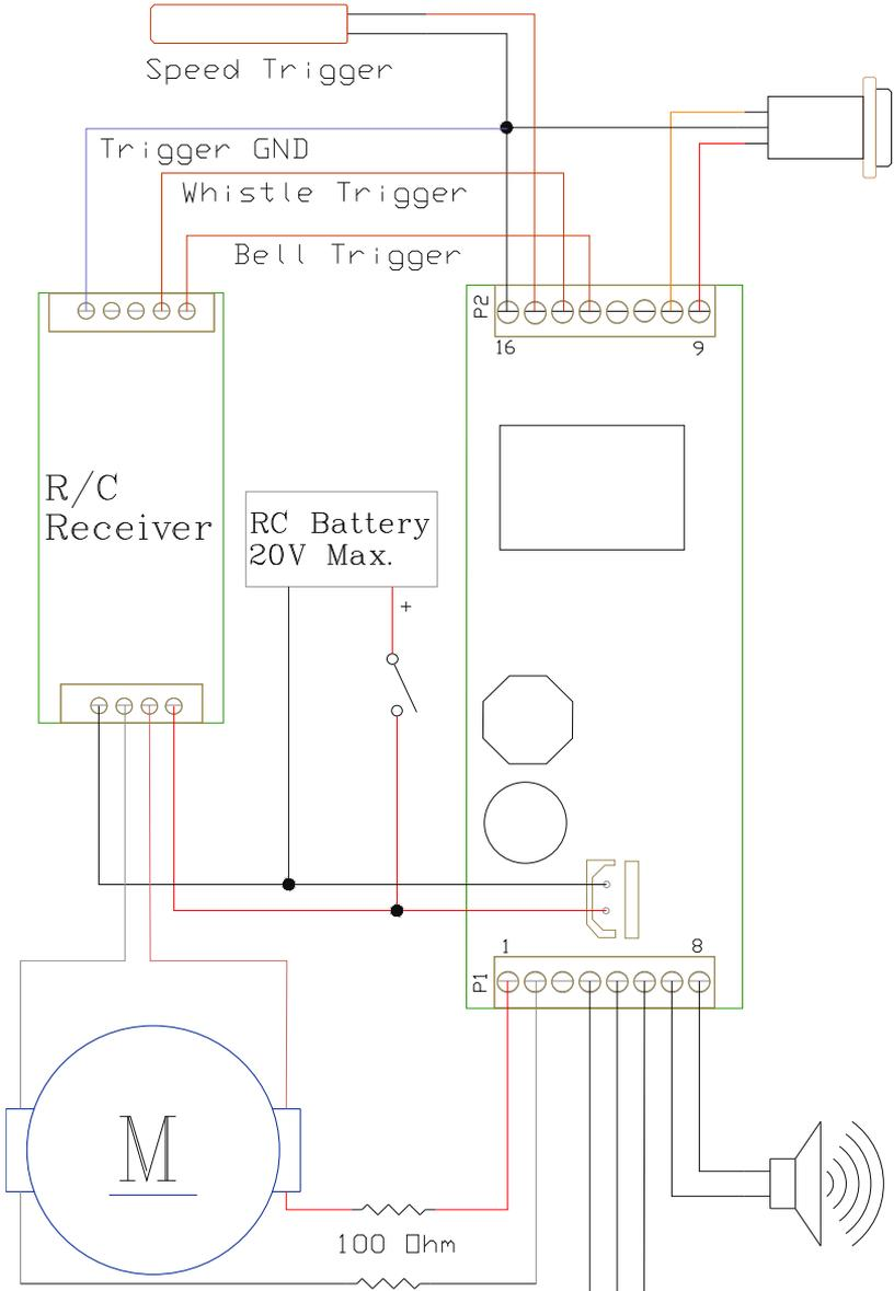
Resistors are optional and suggested. They are not needed if using the 3.6V Battery
