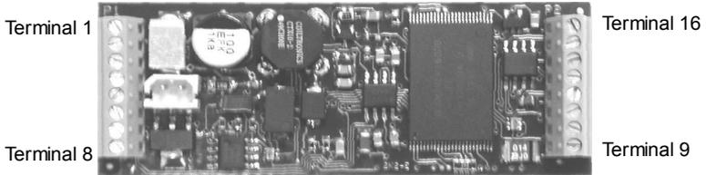
The Terminals, 8 on each end of the board, are numbered 1 through 16. Terminals 1-8 are on the same end as the battery connector. 9-16 are at the opposite end. Terminal 16 is across from terminal 1. The terminals are defined as follows: terminals 10 through 15 are the “trigger” inputs. They are used to cause sounds or effects to occur. Terminal 10 can be used as a trigger input even if the computer access jack is connected
